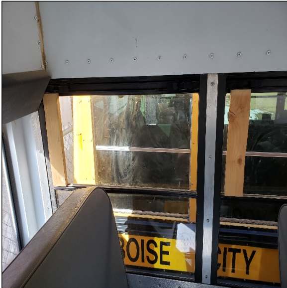
Wood Boards Holding Windows
