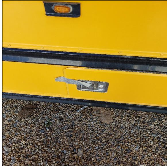
Repair Made with Duct Tape
